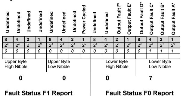
Above each 8,4,2,1 is the corresponding fault for that bit. For instance, above the 8 bit in the Upper byte/Low nibble reads Primary Source, which is the fault .
